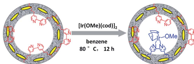
Scheme 3 Synthetic route for the molecular heterogeneous solid catalyst Ir(cod)-BP 0.3 -NT.
