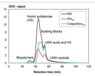
**Fig. 4** Selectivity of pilot-scale SIX® compared to full-scale conventional coagulation and rapid sand filtration analyzed by LC-OCD. LMW = low molecular weight.
