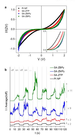
**Fig. 5** Charge transport measurements at the nanoscale, performed by conductive AFM on **Pt NP**, **SA-ZTP**, **SA-ZMPy** and **SA-ZBPy**, at room temperature. (a) *I–V* curves; the curves are normalized at 2 V; inset: magnification of the 0–1 V region. (b) Evolution of the current intensity under light irradiation at a voltage of 2 V; light is successively switched on and off.
