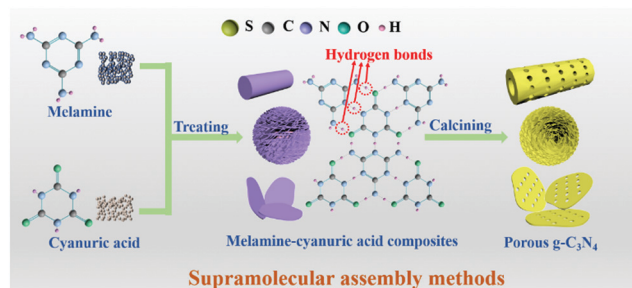
Fig. 7 Schematic illustration of the preparation of porous g-C 3 N 4 (PCN) by supramolecular assembly. In the preparation process, two molecules first formed supramolecular precursors by molecular assembly, then the supramolecular precursors were calcined to form PCN.
