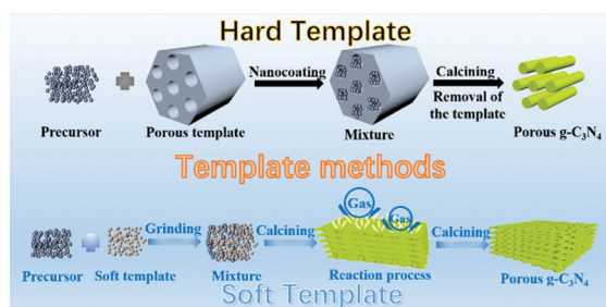
Fig. 3 Schematic illustration of porous g-C 3 N 4 prepared by template methods. The template methods can be divided into two categories: hard template and soft template methods.
