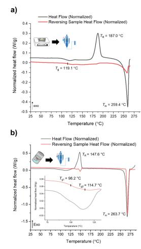
**Fig. 3** mDSC data of (a) SD of polyamorph II obtained by QC; and (b) SD of polyamorph III obtained by BM.
