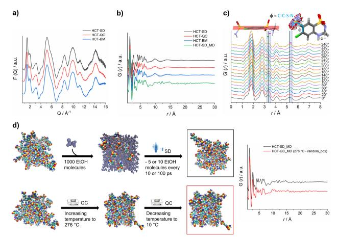
Fig. 4 (a) F(Q) and (b) PDF of experimental HCT polyamorphs and simulated QC method (green curve) with an offset in the *y*-axis for better clarity; (c) simulated PDF of HCT single molecule when varying the dihedral angle  $\Phi$ ; and (d) schematic representation of the MD simulations of both SD and QC methods with the corresponding simulated PDF curves in black and red, respectively (offset in the *y*-axis for better clarity). EtOH stands for ethanol.
