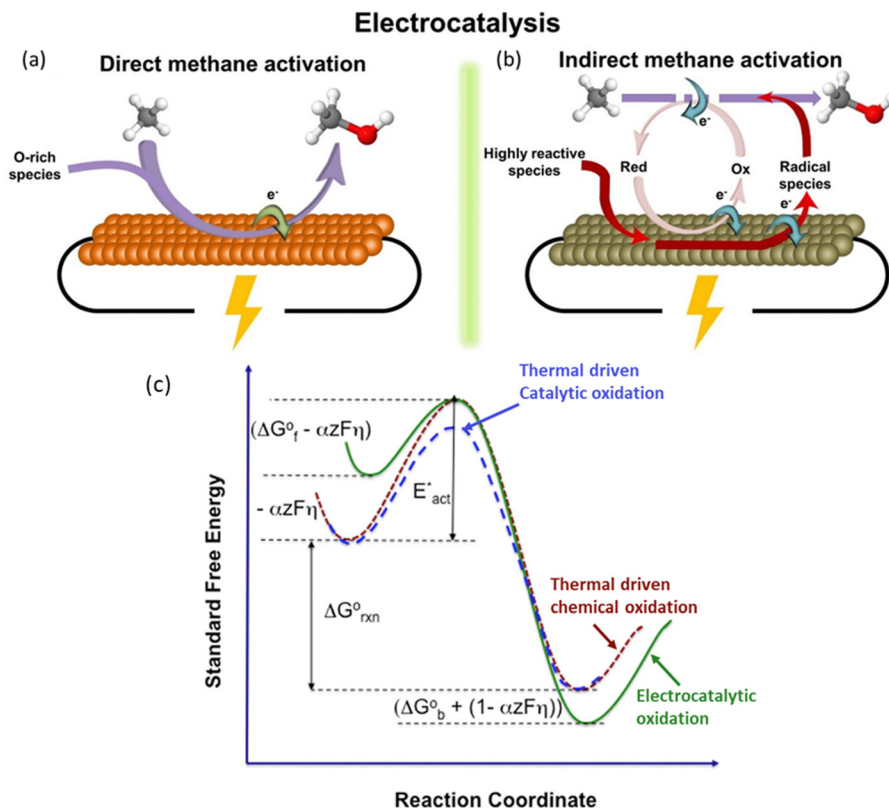
Fig. 4 Schematic illustration of (a) direct electrocatalytic methane activation, and (b) indirect electrocatalytic activation. Reproduced with permission. 15 Copyright 2021, Elsevier. (c) Effects of overpotential on reaction energy profile. Reproduced with permission. 19 Copyright 2016, Elsevier.
