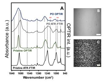
Fig. 1 A) Normalized ATR-FTIR and OPTIR spectra of PET films prior to (pristine) and after exposure at <10% relative humidity. Optical images of film surface in the B) absence and C) presence of saturated relative humidity during exposure. The scale bars for panels B and C are 40  $\mu$ m and 10  $\mu$ m, respectively. The red asterisks (\*\*) represent the vibrational modes observed with ATR-FTIR that were not present in the OPTIR spectra.
