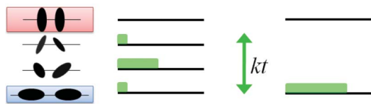
Fig. 7 Description of dichroism ratios R with calculated parameters assuming Boltzmann distribution (2) and a model of energy levels dipole-dipole interactions with their energy interval kT . Blue highlight indicated expansion of equation the number of states ( N 0 or N 90 and green bands in pictures) of directed dipoles and their energy by Boltzmann distribution.
