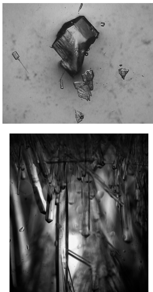
Fig. 1 Crystals of the two forms of compound 1 . Above: orthorhombic form 1o , part of the crystal actually measured (max. linear dimension ca. 0.4 mm). Below: tetragonal form 1t as grown in the test-tube with pentane precipitant (total width ca. 2 mm).
