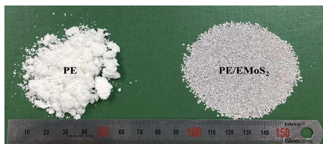
Fig. 3 Optical images of PE and PE/ \text{EMoS}_2 nanocomposites.
