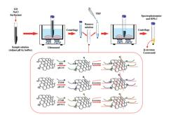
Determination of  $\beta$ -carotene and total carotenoids in fruit juices using surfactant surface decorated graphene oxide based ultrasound-assisted dispersive solid-phase microextraction
