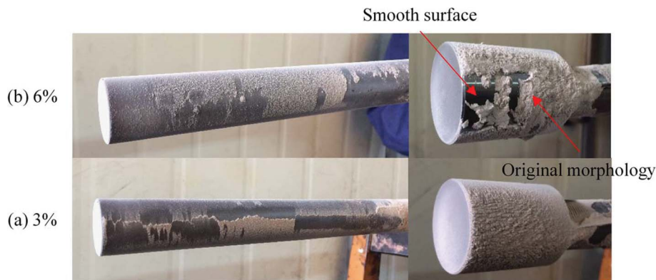
Fig. 13 Macro-morphologies of deposits after the addition of kaolin ( T_{\text{bed}} = 920^\circ\text{C} ).
