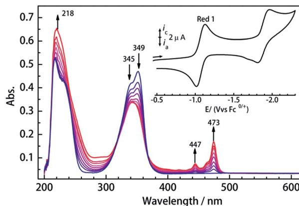
Fig. 2 Changes in the UV/Vis spectrum of **1Dy** during first reduction in  $\text{CH}_2\text{Cl}_2/0.1 \text{ M Bu}_4\text{NPF}_6$  of supporting electrolyte.  $\text{Ag}/\text{Ag}^+$  reference, Pt mesh working, Pt counter electrode. (Insert, cyclic voltammogram of **1Dy** in  $\text{CH}_2\text{Cl}_2/0.1 \text{ M Bu}_4\text{NPF}_6$  measured at 295 K.  $\text{Fc}^{0/+}$  = ferrocene/ferrocenium couple.).
