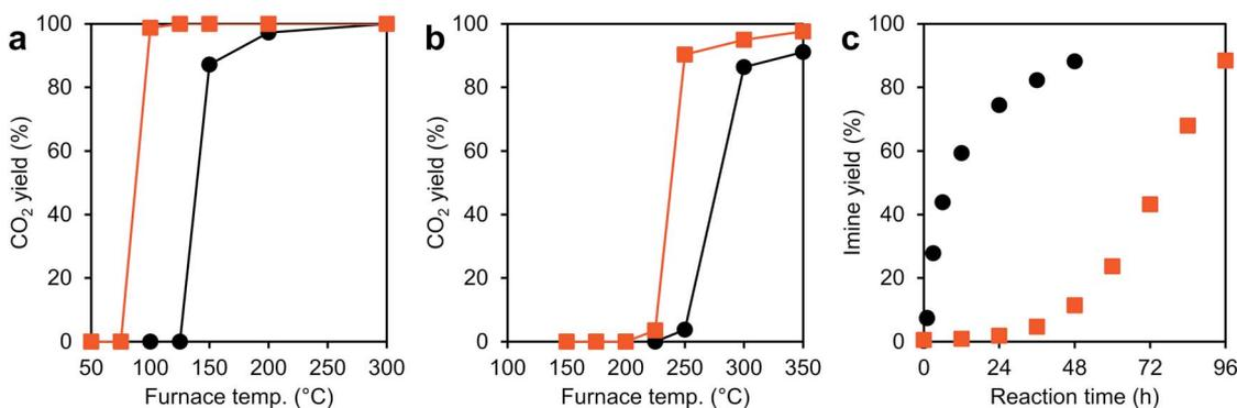
Fig. 4 Results of catalytic reactions with Pt/CeO<sub>2</sub> and CeO<sub>2</sub> catalysts. (a) The vapor-phase CO oxidation reaction catalyzed by Pt/CeO<sub>2</sub>-AN-tEG (red) and Pt/JRC-CEO-5 (black). (b) The vapor-phase CO oxidation reaction catalyzed by CeO<sub>2</sub>-AN-tEG (red) and JRC-CEO-5 (black). (c) The liquid-phase oxidation reaction of benzyl alcohol catalyzed by CeO<sub>2</sub>-AN-tEG (red) and JRC-CEO-5 (black) followed by condensation with aniline.
