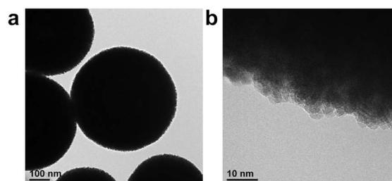
Fig. 3 Morphology of porous ceria sphere (CeO<sub>2</sub>-AN-tEG). (a) TEM image and (b) high resolution TEM image.
