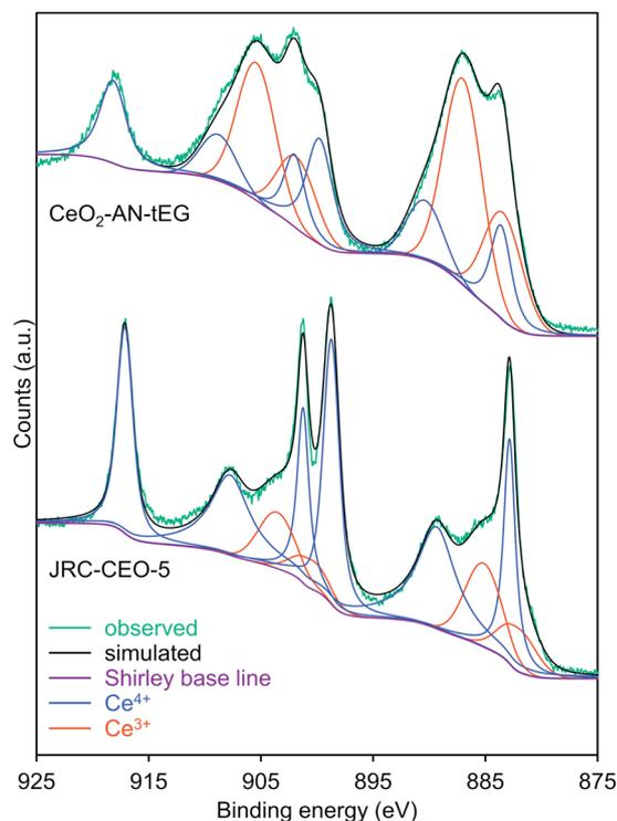
Fig. 5 Ce 3d HAXPES spectra and peak fitting curves of CeO<sub>2</sub>-AN-tEG and JRC-CEO-5. Observed (green), Shirley base line (violet), deconvolution peaks of Ce<sup>4+</sup> (blue), deconvolution peaks of Ce<sup>3+</sup> (red) and simulated curve (black).
