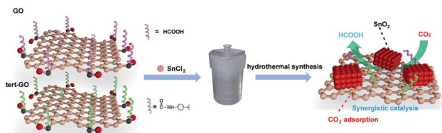
Fig. 1 Synthesis scheme of \text{SnO}_2/\text{GO} and \text{SnO}_2/\text{tert-GO} .
