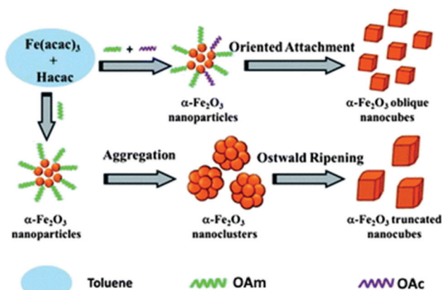
Fig. 11 Scheme depicting the process for the generation of oblique and truncated hematite nanocubes. 56 Copyright 2013, The Royal Society of Chemistry.
