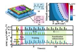
Vertical 0.6 V sub-10 nm oxide-homojunction transistor gated by a silk fibroin/sodium alginate crosslinking hydrogel for pain-sensitization enhancement emulation
