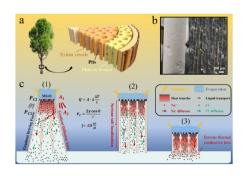
Designing a solar interfacial evaporator based on tree structures for great coordination of water transport and salt rejection
