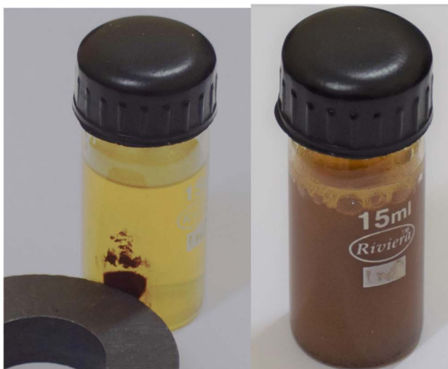
Fig. 11 Regeneration cycles of Co-Al31@Fe 3 O 4 and magnetic separation of the catalyst.
