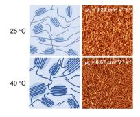
Structural control of charge transport in polymer monolayer transistors by a thermodynamically assisted dip-coating strategy
