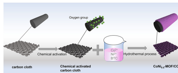
Fig. 1 Schematic illustration of the in situ growth process of \text{CoNi}_{0.5} -MOF on CC.
