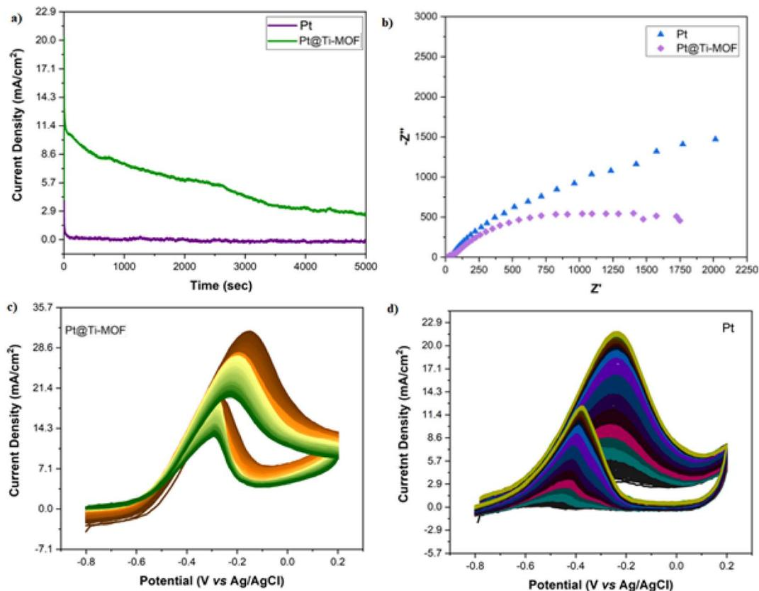
Fig. 6 (a) CA measurement results of the obtained catalysts in 0.5 M KOH buffer solution containing 1 M CH<sub>3</sub>OH at 50 mV s<sup>-1</sup>, (b) Nyquist plots for Pt and Pt@Ti-MOF NPs in 0.5 M KOH buffer solution containing 1 M CH<sub>3</sub>OH, (c) 500 cycles measurement for Pt@Ti-MOF NPs, (d) 500 cycles measurement for Pt NPs.
