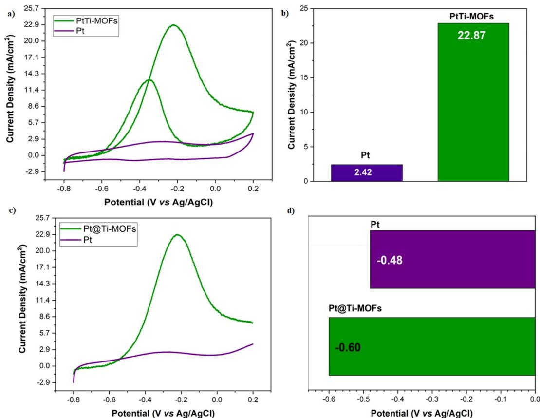
Fig. 4 (a) CV results for Pt and Pt@Ti-MOF NPs in the presence of 0.5 M KOH and 1 M CH<sub>3</sub>OH at a scan rate of 50 mV s<sup>-1</sup>, (b) methanol oxidation peak current density values for Pt and Pt@Ti-MOF NPs, (c) LSV results for Pt and Pt@Ti-MOF NPs in the presence of 0.5 M KOH and 1 M CH<sub>3</sub>OH at 50 mV s<sup>-1</sup> scan rate, (d) methanol oxidation onset potential values for Pt and Pt@Ti-MOF NPs.
