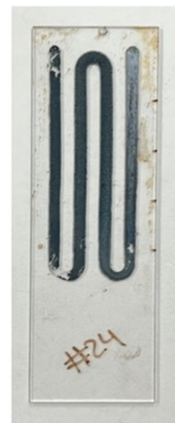
Fig. 10 XRD scan of annealed \text{Sb}_2\text{S}_3 thin films at 300 °C for 60 min on glass substrate. GSAS 2 refined XRD data (left); photo image of annealed sample (right).
