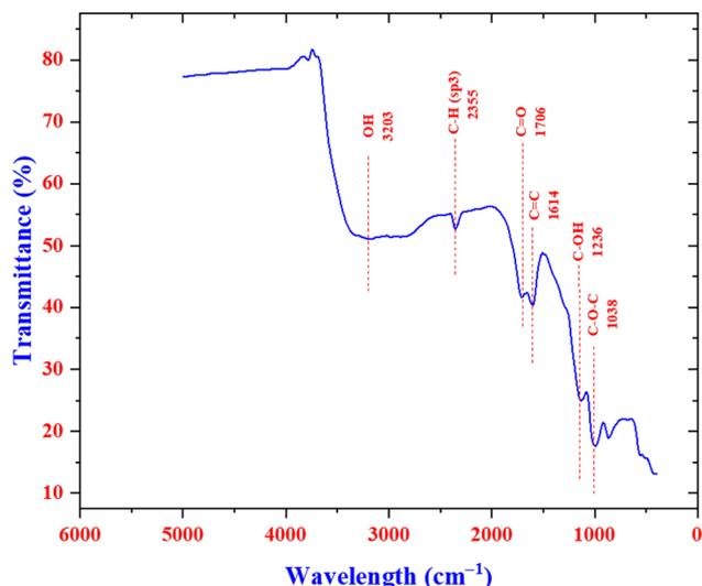
Fig. 5 FTIR spectra of graphene.
