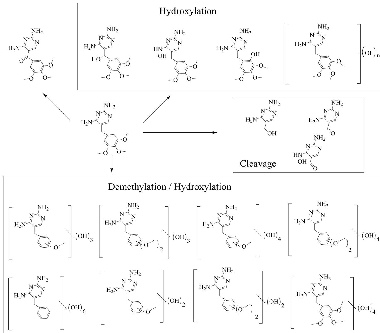
**Figure 7.** Two major processes (Demethylation and hydroxylation) involved in the direct photolysis mechanism of TMP.<sup>129</sup> Redrawn with permission from Ref. 129. © 2010 Elsevier Ltd.
