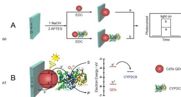
**Scheme 1** (A) Fabrication of the photocatalysts and photoelectrodes. (B) Illustration of the electron transfer steps of the CYP2C9/QDs/ITO electrode upon irradiation.
