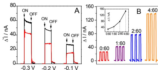
**Fig. 1** (A) Photocurrent responses at potentials of -0.1, -0.2 and -0.3 V on the QDs/ITO (in red) and CYP2C9/QDs/ITO (in black) (CYP2C9:QDs ratio of 1:60) electrodes upon the illumination of white light. (B) Photocurrent responses on the CYP2C9/QDs/ITO electrode at -0.2 V with different molar ratios of CYP2C9 to QDs.
