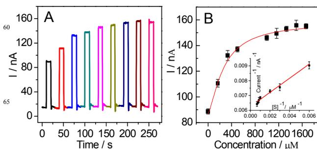
**Fig. 2** (A) The cathodic photocurrents on the CYP2C9/QDs/ITO electrode (CYP2C9:QDs ratio of 2:60) in air-saturated 0.1 M pH 7.4 PBS with successive addition of tolbutamide at the applied potential of -0.2 V. (B) Calibration plots illustrating the electrode response to tolbutamide addition. Insert: double-reciprocal plot of the photocurrents and the concentrations of tolbutamide.
