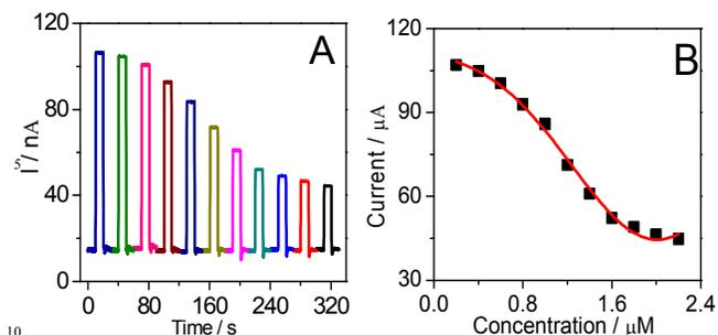
**Fig. 3** (A) Analysis of the inhibition effect on 4-hydroxylation of tolbutamide by sulfaphenazole. The cathodic photocurrents at  $-0.2$  V on the CYP2C9/QDs/ITO electrode (CYP2C9:QDs ratio of 2:60) by varying sulfaphenazole concentrations in  $0.1$  M pH  $7.4$  PBS containing  $75$   $\mu$ M tolbutamide. (B) Changes in bioelectrocatalytic currents at  $-0.2$  V upon addition of sulfaphenazole.
