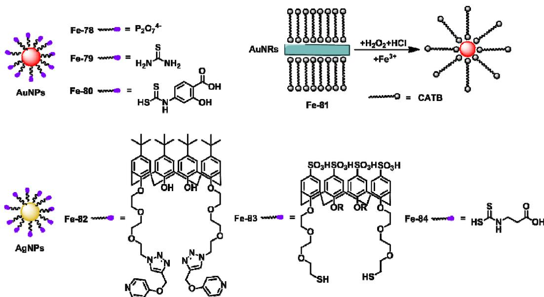
Next, a few examples of colorimetric Fe<sup>3+</sup> sensors based on AuNPs will be discussed. Wu *et al*<sup>175</sup> have introduced a selective colorimetric Fe<sup>3+</sup> detection method using pyrophosphate (P<sub>2</sub>O<sub>7</sub><sup>4-</sup>) functionalized AuNPs (**Fe-78**). The absorbance of **Fe-78** at 535
