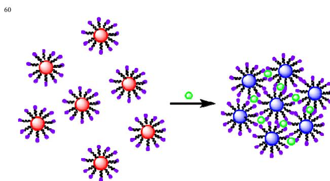
**Scheme 1** Schematic depiction of AuNP-based colorimetric assays for metal ions.
