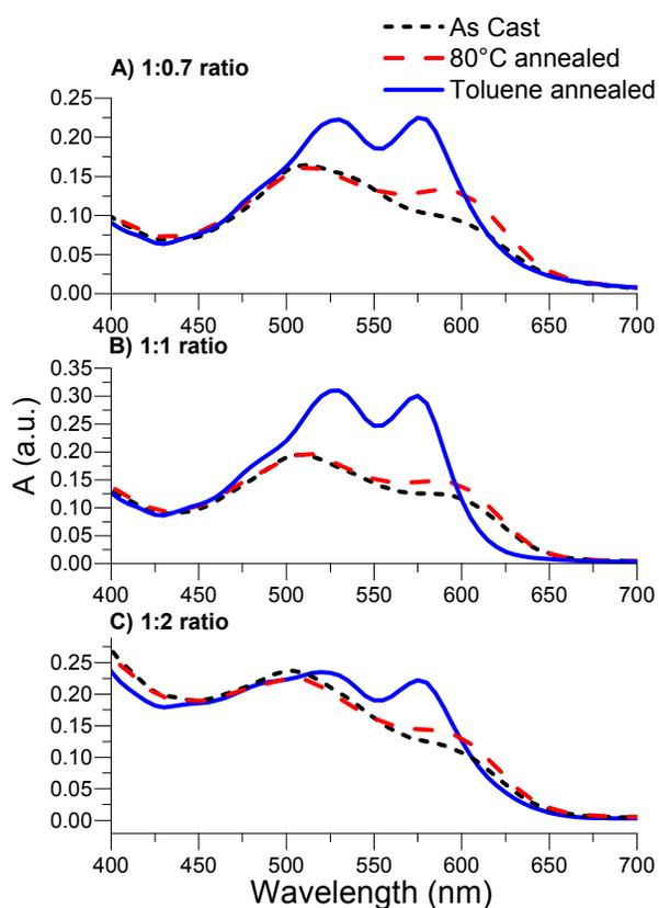
Fig. 9 UV-vis film absorption of compound **1** at different ratio of PC<sub>61</sub>BM with different annealing conditions
