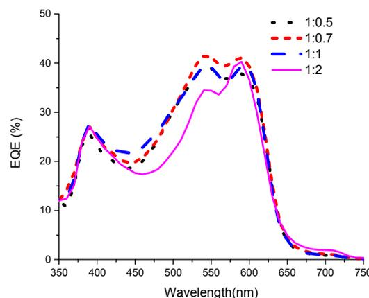
**Fig. 8** EQE for **3**:PC<sub>61</sub>BM at different D/A ratios after toluene annealing
