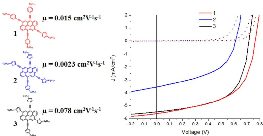
Novel anthanthrene derivatives have been tested as *p*-type materials in bulk-heterojunction organic solar cells and organic field-effect transistors.
