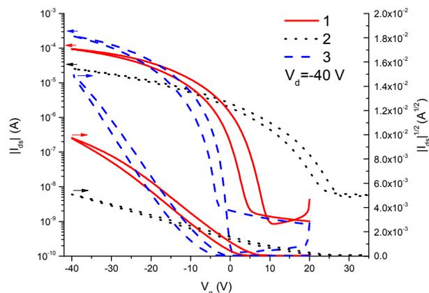
**Fig. 5** Transfer characteristics after cyclohexane solvent annealing for compound **1** and toluene annealing for compound **2** and **3**
