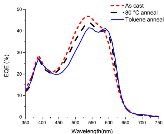
**Fig. 7** EQE for **3**:PC<sub>61</sub>BM at a ratio of 1:0.7 with different treatments
