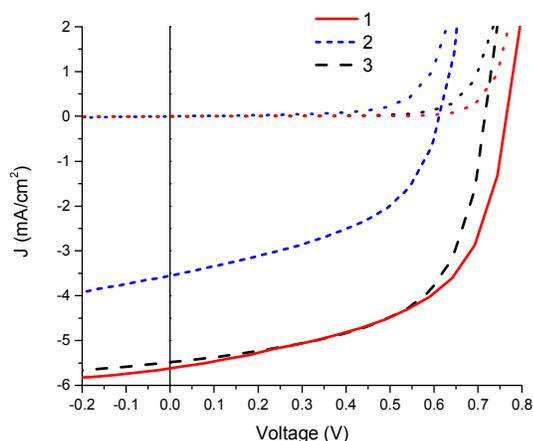
**Fig. 6** J-V curves for compounds **1** (as cast), **2** (80°C annealed) and **3** (toluene annealed) at a D/A ratio of 1:0.7 under illumination and dark (short dotted lines) under the optimized conditions reported in bold in
