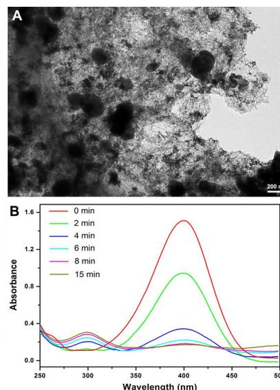
**Fig. 10.** TEM image of rGO/Fe<sub>3</sub>O<sub>4</sub>/Au composite using GO only to anchor Fe<sub>3</sub>O<sub>4</sub> and Au (A). UV-vis spectra of the catalytic reduction of 4-NP to 4-AP developed at different reaction times for the sample (B).
