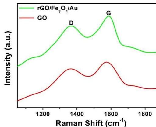
**Fig. 2.** Raman spectra of the pristine GO sheets and rGO/Fe<sub>3</sub>O<sub>4</sub>/Au composite.
