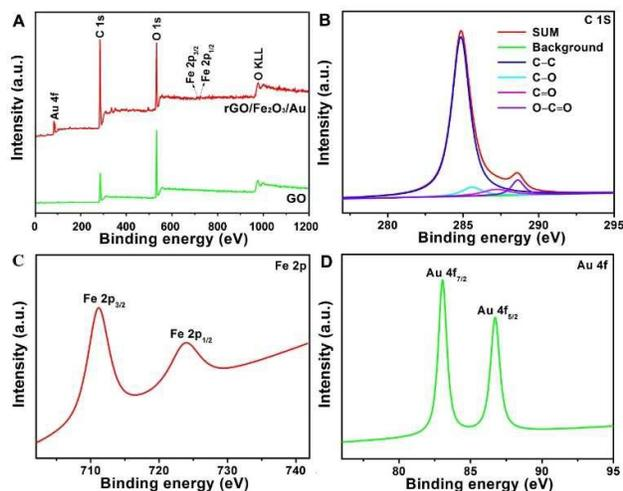
**Fig. 3.** XPS spectra of the pure GO sheets and as-prepared rGO/Fe<sub>3</sub>O<sub>4</sub>/Au composite. XPS survey spectra (A), C1s spectrum of rGO/Fe<sub>3</sub>O<sub>4</sub>/Au (B), Fe 2p spectrum of rGO/Fe<sub>3</sub>O<sub>4</sub>/Au composite (C) and Au 4f spectrum of the rGO/Fe<sub>3</sub>O<sub>4</sub>/Au composite (D).
