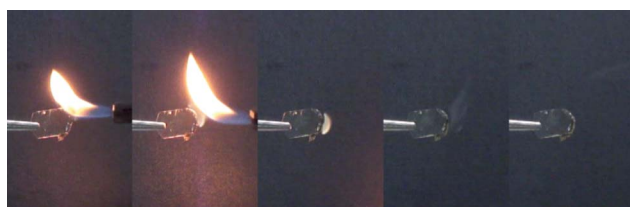
Fig. 4 Flammability of PU prepared by reacting PPDI with the PPC-diol prepared using phenylphosphonic acid as the chain-transfer agent (entry 15). The pictures were taken at 0.8 second intervals from a video clip.
