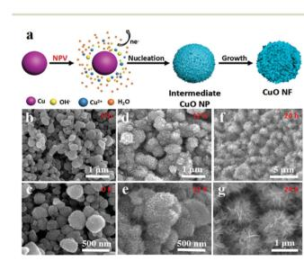
**Fig. 3** (a) Schematic formation of CuO NFs; (b and c) SEM images of CuO NP/CF at the beginning of the NPV step; (d and e) SEM images of the CuO NP/CF after conducting the NPV step in 1.0 M KOH solution for 10 hours; (f and g) SEM images of the CuO NF/CF after the NPV step in 1.0 M KOH solution for 24 hours.
