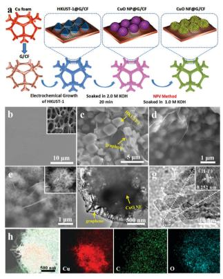
Fig. 1 (a) Schematic illustration of the *in situ* fabrication procedure for CuO NF@G/CF. (b) SEM image of G/CF (inset: SEM image of G/CF at low magnification); (c-e) SEM images of HKUST-1@G/CF, CuO NP@G/CF and CuO NF@G/CF, respectively; (f and g) TEM and HR-TEM images of CuO NF@G/CF; (h) elemental mapping of CuO NF@G/CF.
