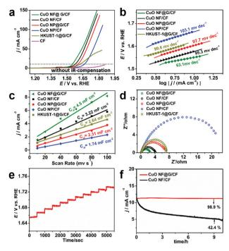
**Fig. 4** (a–d) LSV curves, Tafel plots,  $C_{dl}$  plots and EIS data of CuO NF@G/CF, CuO NP@G/CF, CuO NF/CF, CuO NP/CF, HKUST-1@G/CF and pristine CF, respectively; (e) multi-current process of CuO NF@G/CF in 1.0 M KOH solution; (f) chronopotentiometric durability test of CuO NF@G/CF.
