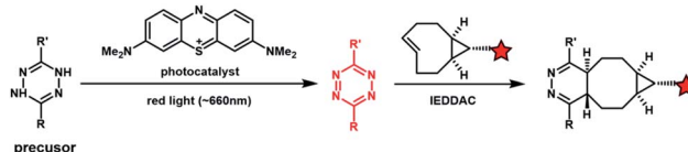
Fig. 4 Photocatalytic activation of the IEDDAC reaction.
