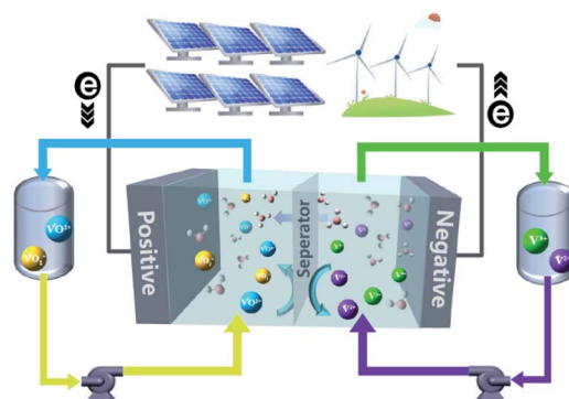
Fig. 1 A schematic diagram of a VFB.
