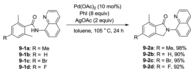
Scheme 11 Synthesis of isoindolinones with PhI.
