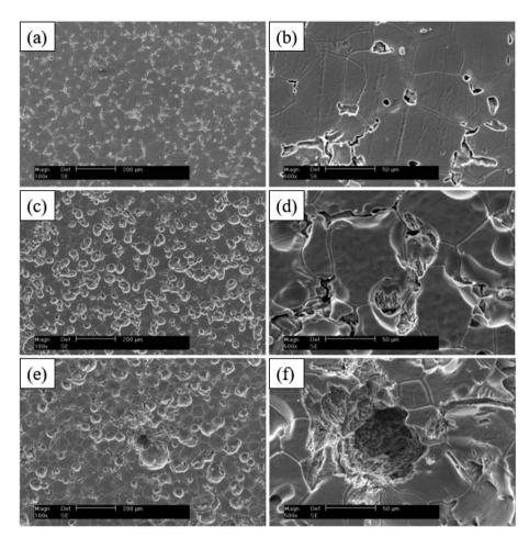
Fig. 8 SEM corrosion morphology of cast Mg alloy GW93 immersed in 3.5% NaCl for 30 min (a and b); 48 h (c and d); 72 h (e and f).<sup>110</sup>
