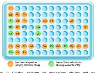
Fig. 17 Suitable elements for magnesium alloying and their applications.  $^{\rm 191-193}$
