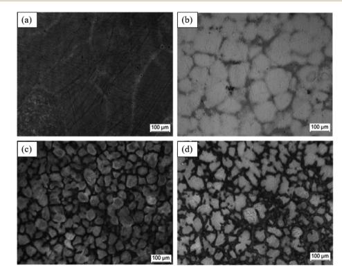
Fig. 20 Optical microstructure changes of Mg–Zn alloys (a) pure Mg, (b) Mg–1Zn, (c) Mg–5Zn and (d) Mg–7Zn.<sup>214</sup>
