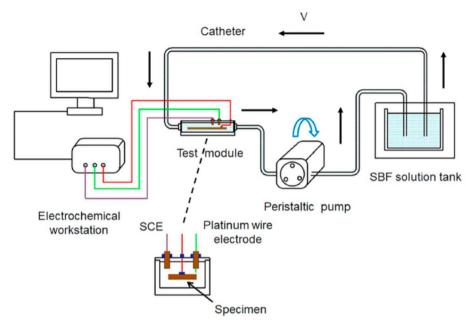
Fig. 16 Schematic diagram of a dynamic flow field test device.<sup>181</sup>
