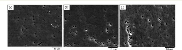
Fig. 18 SEM images of the (a) Mg-0.54Ca alloy; (b) Mg-0.79Ca alloy; (c) Mg-1.35Ca alloy.<sup>198</sup>
