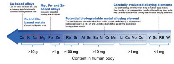
Fig. 2 Contents of metal elements in human body and suggestions on alloying of each element.<sup>51</sup>
