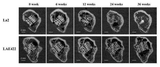
Fig. 3  $\mu$ CT images of longitudinal sections of La2 and LAE422 degradation evolution at 36 weeks.<sup>60</sup>
