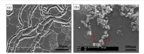
Fig. 10 Typical filamentary corrosion morphologies of Mg–3Zn immersed in 0.01 mol per L NaCl solution for 6 h at different scales (50 μm and 200 μm).<sup>121</sup>
