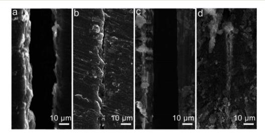
Fig. 29 SEM images of the (a) scratched SHEP coating, (b) healed SHEP coating, (c) healed PF-POS@silica coating, and (d) healed SHEP/PF-POS@silica coating.<sup>271</sup>
