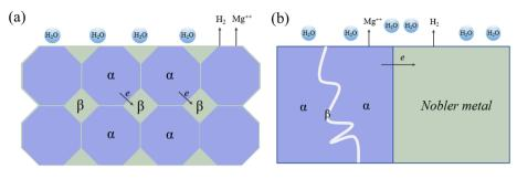
Fig. 6 (a) Schematic of internal micro-galvanic corrosion. (b) External galvanic corrosion.<sup>131</sup>
