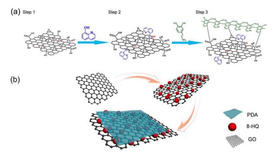
Fig. 24 (a) The synthesis process of sandwich-like GO/8-HQ/PDA structures and (b) schematic illustration of the synthesis of the GO/8-HQ/PDA.<sup>244</sup>
