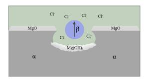
Fig. 7 Schematic of pitting corrosion.131
