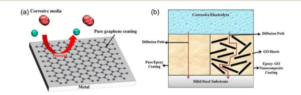
Fig. 22 (a) The graphene anti-corrosion coating.<sup>234</sup> (b) the "labyrinth effect" of GO enhanced epoxy resin coating.<sup>235</sup>
