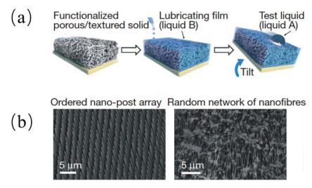
Fig. 30 (a) Schematic diagram of SLIPS assembly process; (b) SEM: an epoxy-resin-based nanofabricated post array (left) and a Teflon-based porous nanofibre network (right).<sup>272</sup>
