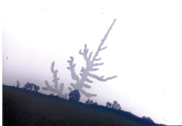
Fig. 2 Dendritic growth of lithium during its electrodeposition. Reprinted with permission from R. R. Chianelli, J. Cryst. Growth , 1976, 34 , 239–244. Copyright 1976 Elsevier.
