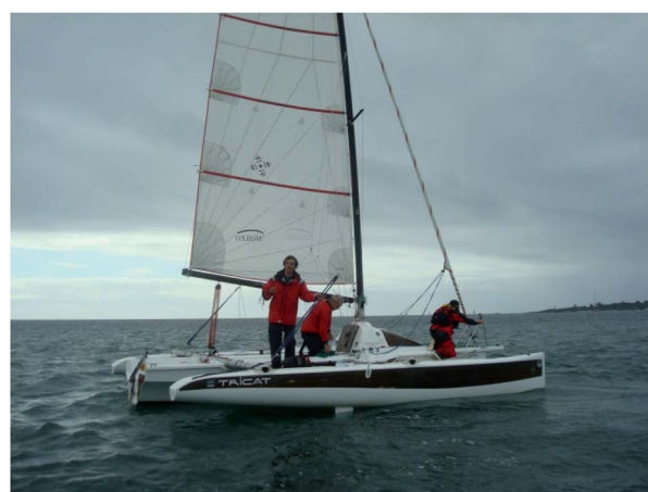
Fig. 3 Gwalaz, flax fibre reinforced trimaran.
