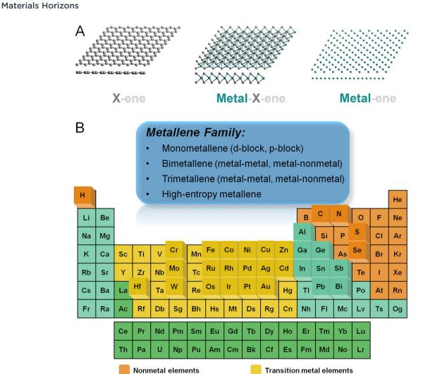
Fig. 1 (A) Schematic illustration showing three-generational development of 2D atomically thin materials including metal-free (X-ene, X = B, C, N, P, etc.), transition metal compounds (metal-X-ene, X = C, N, O, S, etc.), and metallic materials (metal-ene). (B) Overview of the elements involved in metallenes in the periodic table achieved by either experiments or theoretical calculations. (A) Reproduced from ref. 8 with permeation from CellPress. Copyright 2019
