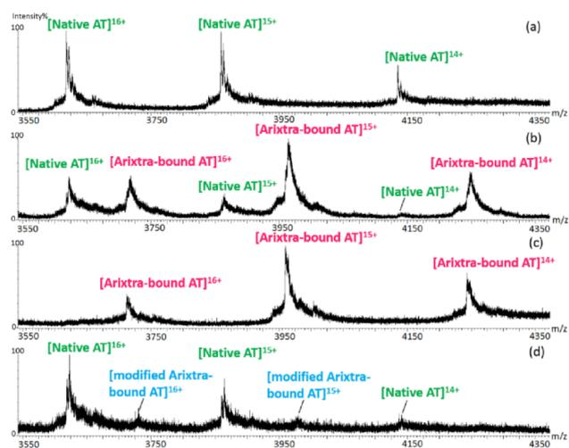
**Figure 2** Electrospray ionization mass spectra, obtained under non-denaturing conditions, of (a) ATIII; (b) ATIII incubated with Arixtra for 1h; (c) ATIII incubated with Arixtra for 12h; (d) ATIII incubated with the Arixtra-like hexasaccharide, minus 3-O-sulfation, for 12h.
