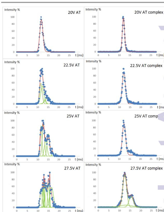
**Figure 7** Experimental drift time distributions (ms) of +15 charge state of ATIII (left panels) and ATIII-Arixtra complex (right panels) as a function of trapping CE varying from 20V to 27.5V in 2.5 V increments. The normalized experimental drift time distribution is shown by the blue dots. The fit of the data to a series of Gaussian distributions is shown in green, and the sum of the component Gaussians is shown in red.
