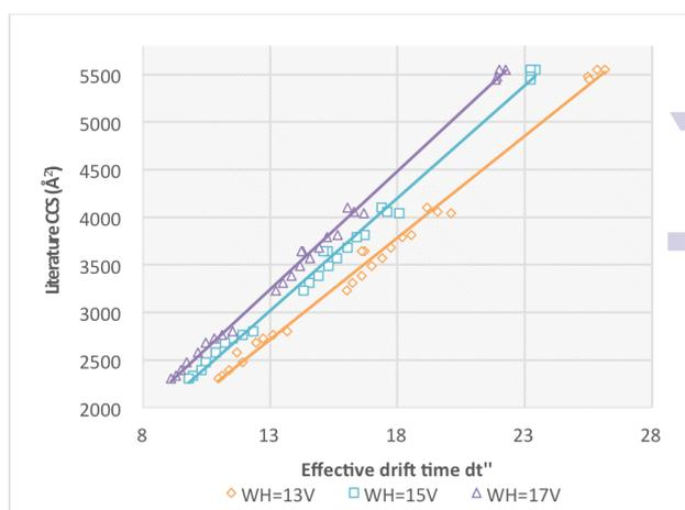
**Figure 1** The calibration curves were constructed at three wave heights combining data from cytochrome c, myoglobin, avidin, BSA and concanavalin A, displayed as literature CCS vs effective drift time for each charge state.
