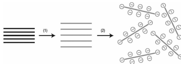
Fig. 1 Scheme showing a chemical route to the synthesis of aqueous GO suspension: (1) oxidation of graphite (black blocks) to graphite oxide (lighter coloured blocks) with a greater interlayer distance; (2) exfoliation of graphite oxide in water by sonication to obtain GO suspensions that are stabilized by electrostatic repulsion. Reprinted with permission from Macmillan Publishers Ltd: [Nature Nanotechnology] (ref. 95), copyright (2008).
