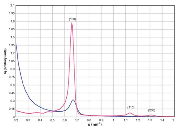
Fig. 3 SAXS data for the SBA-15  $\text{SiO}_2$  precursor (red) and the mesoporous product (blue) showing retention of the mesoporous order of the precursor in the product phase.
