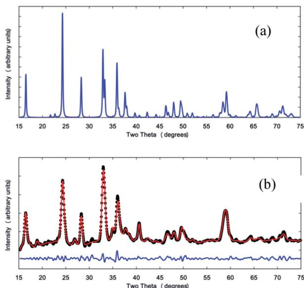
Fig. 4 (a) A simulated X-ray diffraction pattern of  $\text{Li}_2\text{MnSiO}_4$  (b) Rietveld refinement results of structural models with the powder XRD pattern of the mesoporous Mn-deficient product phase. Black dots represent the experimental data, the model is the red line through the data and the blue line below is the difference between the model and the data.
