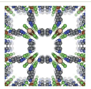
Fig. 1 The crystal structure of SIFSIX-3-Fe viewed down the c-axis, which we define by the metal-SiF<sub>6</sub> chain. Colors = {blue: N, gray: C, white: H, green: F, orange: S, tan: Fe}.
