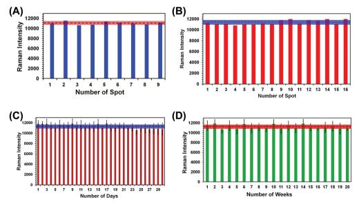
Fig. 4 Histograms of SERS intensity of TNT at 1380 cm<sup>-1</sup> collected from (A) 9 randomly selected spots on a particular nanosensor; (B) four randomly selected areas of four different nanosensors (1-4, 5-8, 9-12, and 13-16), which were prepared from four different batches of Au TNPs; (C) one SERS nanosensor over an entire month; (D) 20 individual nanosensors over the course of 5 months. The error bars in (C) and (D) represent measurements from six spots each.
