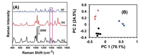
Fig. 3 (A) Representative SERS spectra acquired using the nanosensor from 100 fM: (a) TNT, (b) TNB, and (c) DNT at 1380 cm<sup>-1</sup> (purple box). Scale bar represents counts per second. (B) Plot of PCA scores for SERS at 100 fM concentration of TNT (blue spheres), TNB (red triangles), and DNT (black square). DA classified 100% of spectra correctly. Here n = 18, DA prediction 100%.
