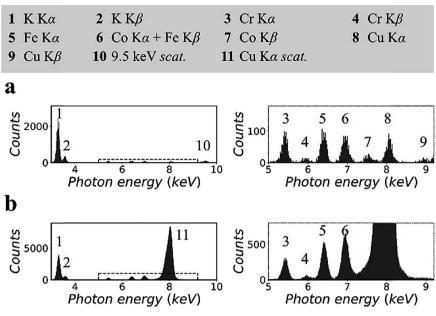
Fig. 2 X-ray fluorescence spectra of the lithium borate pellet that includes 100 ppm chromium, iron, cobalt, and copper: (a) measured in the synchrotron polarized experiment and (b) measured in the laboratory unpolarized experiment. Details of spectra were enlarged and attached on the right side.
