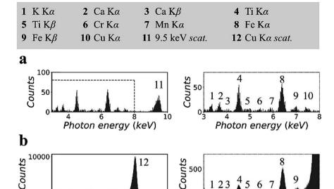
Fig. 3 X-ray fluorescence spectra of the CRM, NIST 81a, glass sand. The original material was mixed with a cellulose matrix at a mass fraction of 30%: (a) measured in the synchrotron polarized experiment and (b) measured in the laboratory unpolarized experiment. Details of spectra were enlarged and attached on the right side.
