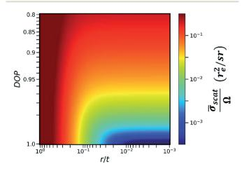
Fig. 4 Average scattering cross section  $\bar{\sigma}_{\rm scat}$  with respect to the DOP of primary X-rays and the ratio of capillary radius r to collimator plate thickness t. Scattering cross section is in the units of  $r_{\rm e}^2$ , where  $r_{\rm e}$  denotes the classical electron radius and equals  $2.82 \times 10^{-5}$  Å, and is normalized by the effective solid angle  $\Omega$  of capillaries.
