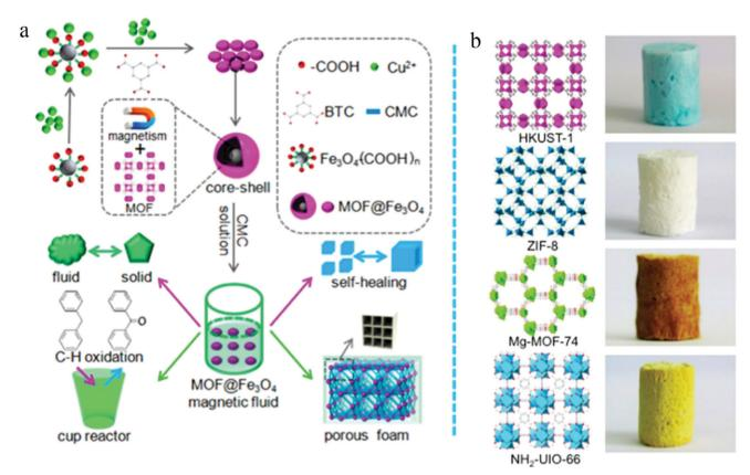
Fig. 24 (a) Schematic procedure for producing HKUST-1@Fe<sub>3</sub>O<sub>4</sub>-MF and its transformation from magnetic fluid to gel, shaped bodies, and a porous foam. (b) Other foams derived from representative MOFs through this strategy
