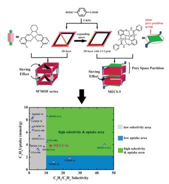
Fig. 22 Imitating M'MOF to design an MOF with high C<sub>2</sub>H<sub>2</sub>/C<sub>2</sub>H<sub>4</sub> selectivity and C<sub>2</sub>H<sub>2</sub> uptake
