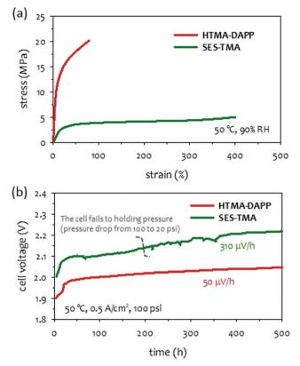
Fig. 16 (a) Stress–strain curves of HTMA-DAPP and SES-TMA AEMs. (b) Comparison of long-term performance of AEMWEs using HTMA-DAPP (78  $\mu$ m thick) and SES-TMA (53  $\mu$ m thick) AEMs. Ionomer: Aemeon, Co<sub>3</sub>O<sub>4</sub> (3 mg cm<sup>-2</sup>), cathode: Pt black (3 mg<sub>Pt</sub> cm<sup>-2</sup>). The AEMWE cell data was produced at Nel Hydrogen.
