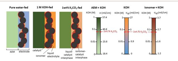
Fig. 3 Schematic illustration of a half cell with supplying pure water, 1 M KOH, or 1 wt%  $K_2CO_3$  solution.<sup>12</sup> We estimated the conductivity of AEM from the high-frequency resistance of the cell using an HTMA-DAPP AEM as a function of KOH concentration at 50 °C.
