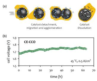
**Fig. 15** (a) Catalyst degradation pathways under AEMWE operating conditions. (b) Durability of 1 M KOH-fed AEMWE at 500 mA cm<sup>-2</sup> at 45 °C. AEM: Sustainion<sup>®</sup> X37-50, anode: CuCo-oxide on nickel form (CE-CCO), cathode: Pt/C (1 mg<sub>Pt</sub> cm<sup>-2</sup>).<sup>92</sup> Adapted with permission.<sup>92</sup> Copyright 2020, Elsevier.
