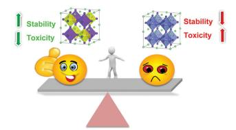
Scheme 2 Differences between lead-free double perovskites and lead halide perovskites
