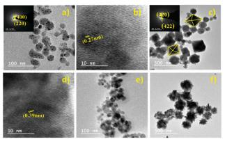
Fig. 11 Cs<sub>2</sub>AgBiCl<sub>6</sub> MCs: (a) TEM image (SAED pattern inset) and (b) HRTEM image in organic medium and (c) TEM image (SAED pattern inset) and (d) HRTEM image in aqueous medium. Cs<sub>2</sub>AgBiBr<sub>6</sub> MCs: TEM images in (e) organic medium and (f) aqueous medium. Reproduced with permission.<sup>76</sup> Copyright 2021, Elsevier.
