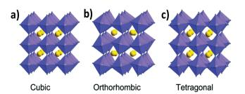
Fig. 1 Different crystal structures of metal halide perovskites: (a) cubic, (b) orthorhombic and (c) tetragonal. Reproduced with permission.<sup>26</sup> Copyright 2019, Royal Society of Chemistry.
