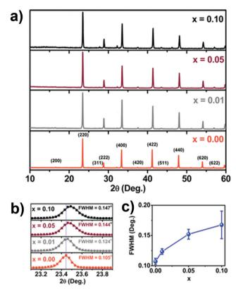
Fig. 5 (a) XRD patterns of undoped and Cu doped Cs<sub>2</sub>AgSbCl<sub>6</sub> MCs, (b) expansion of the (220) plane in the XRD patterns and (c) broadening of the FWHM. Reproduced with permission. 80a Copyright 2018, American Chemical Society.
