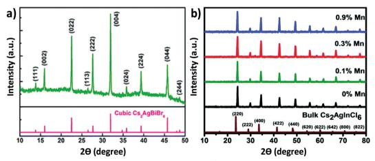
Fig. 4 XRD pattern of (a) the Cs<sub>2</sub>AgBiBr<sub>6</sub> thin film. Reproduced with permission.<sup>73</sup> Copyright 2018, Royal Society of Chemistry. XRD patterns of (b) undoped and Mn doped Cs<sub>2</sub>AgInCl<sub>6</sub> double perovskite MCs. Reproduced with permission. <sup>78</sup> Copyright 2018, Royal Society of Chemistry.
