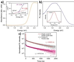
Fig. 7 (a) Absorption spectra, (b) PL spectra and (c) PL decay curves of  $Cs_2AgBiBr_6$  double perovskite MCs respectively. Reproduced with permission. <sup>72</sup> Copyright 2016, American Chemical Society.
