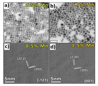
Fig. 13 TEM images of (a) 0.5% and (b) 1.5% and HRTEM images of (c) 0.5% and (d) 1.5% Mn-doped Cs<sub>2</sub>AgInCl<sub>6</sub> NCs respectively. Reproduced with permission.<sup>84</sup> Copyright 2018, American Chemical Society.
