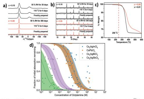
Fig. 16 (a) NMR, (b) P-XRD and (c) TGA spectra of undoped and Cu doped  $Cs_2AgSbCl_6$  MCs. Reproduced with permission. Reproduced with permission. Chemical Society. (d) Stability analysis of Cs<sub>2</sub>AgSbCl<sub>6</sub>, Cs<sub>2</sub>AgInCl<sub>6</sub>, Cs<sub>2</sub>AgBiCl<sub>6</sub> and CsPbCl<sub>3</sub> NCs by amine titration. Reproduced with permission. 83 Copyright 2019, American Chemical Society.
