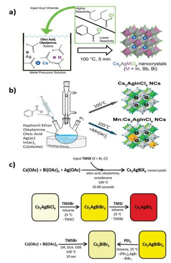
Fig. 6 Synthesis of (a) metal halide double perovskite nanocrystals. Reproduced with permission.<sup>83</sup> Copyright 2019, American Chemical Society. Synthesis of (b) undoped and Mn doped Cs<sub>2</sub>AgInCl<sub>6</sub> nanocrystals. Reproduced with permission.<sup>84</sup> Copyright 2018, American Chemical Society. (c) Cs<sub>2</sub>AgBiX<sub>6</sub> nanocrystals via an anion exchange method. Reproduced with permission.<sup>86</sup> Copyright 2018, American Chemical Society.
