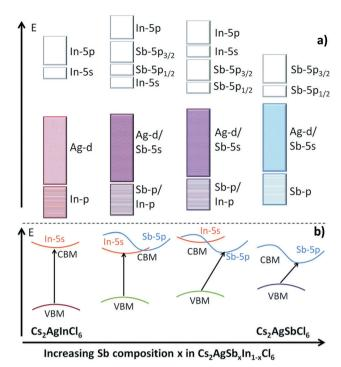
Fig. 10 (a) Schematic diagram of the bonding and antibonding orbitals of Cs<sub>2</sub>AgSb<sub>x</sub>In<sub>1-x</sub>Cl<sub>6</sub> and (b) transition from direct to indirect bandgaps on changing the character of the VBM and CBM. Reproduced with permission.90 Copyright 2017, Royal Society of Chemistry.
