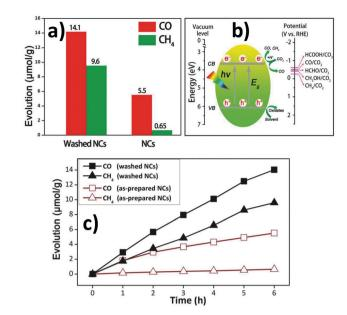
Fig. 20 (a) Comparison of the performance of CO<sub>2</sub> reduction between the as-prepared and washed Cs<sub>2</sub>AgBiBr<sub>6</sub> nanocrystals, (b) photo-reduction of CO<sub>2</sub> on the surfaces of the nanocrystals, and (c) time courses of CO and CH<sub>4</sub> evolution. Reproduced with permission. <sup>103</sup> Copyright 2018, Wiley-VCH.
