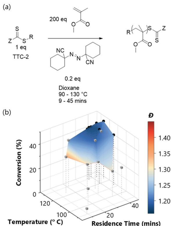
**Fig. 6** (a) Scheme and (b) multi-objective optimisation (TSEMO algorithm) for the RAFT polymerisation of methyl methacrylate using TTC-2 as the RAFT agent and ACHN as the initiator ([MMA] : [TTC-1] : [ACHN] 200 : 1 : 0.2). The LHC and TSEMO experiments are differentiated – LHC – grey cubes, TSEMO – black circles.
