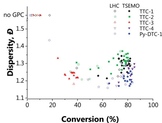
Fig. 3 The property space (in terms of conversion and dispersity) for each of the five RAFT agents used for the RAFT polymerisation of *tert*-butylacrylamide ([monomer] : [CTA] : [initiator] 200 : 1 : 0.1). [Condition limits: 4–20 min, 80–120 °C.]
