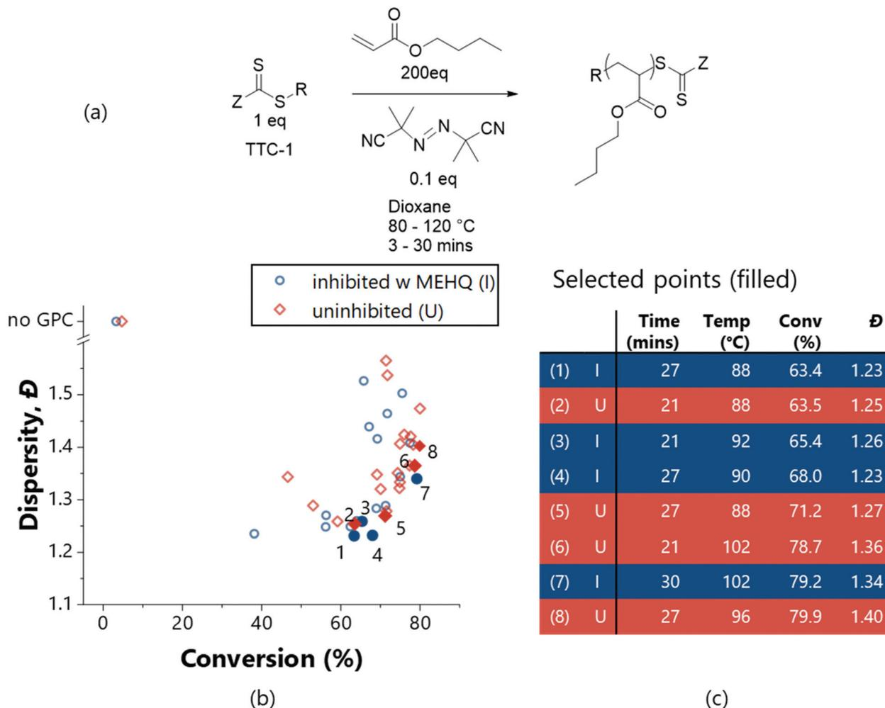
**Fig. 5** Multi-objective optimisations (TSEMO algorithm) for the RAFT polymerisation of *n*-butyl acrylate (scheme in (a)) inhibited (I – blue circles) and uninhibited (U – red squares), using TTC-1 as the RAFT agent and AIBN as the initiator, in dioxane ([monomer] : [CTA] : [initiator] 200 : 1 : 0.1, 30% w/w). [Condition limits: 3–30 min, 80–120 °C.] The full data for selected points (filled and numbered in (b)) are given in (c). For surfaces and all experimental data see ESI.†
