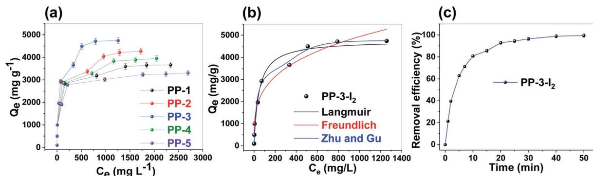
Fig. 5 Iodine adsorption study in *n*-hexane: (a) adsorption isotherms of different porous polymers, (b) Langmuir, Freundlich and Zhu and Gu adsorption isotherm models for PP-3, and (c) iodine adsorption kinetics.
