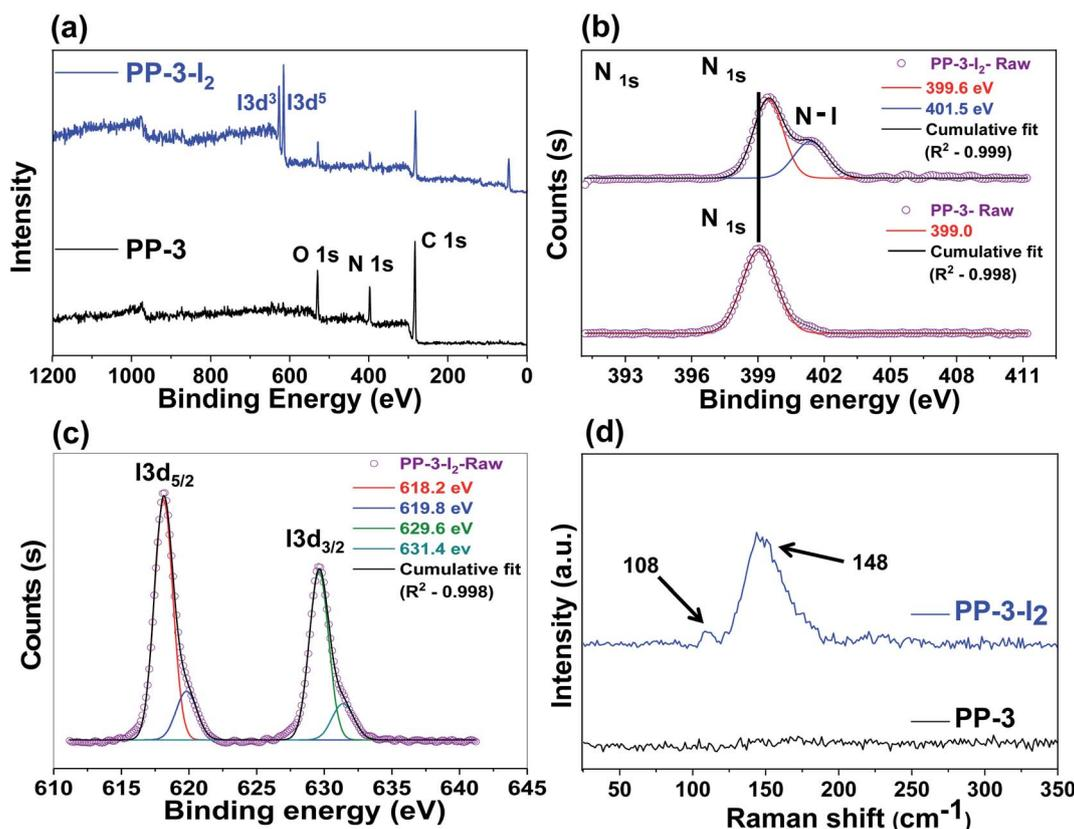
Fig. 8 XPS survey spectra of PP-3 and PP-3-I<sub>2</sub> (a) full spectra, (b) N 1s, (c) I 3d, and (d) Raman spectra analysis.
