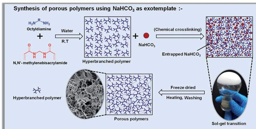
Scheme 1 Synthesis of porous polyaminoamides using  $\text{NaHCO}_3$  as the exotemplate.
