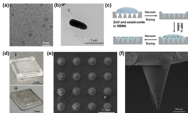
**Fig. 2** (a) TEM image of ZnO NPs. (b) TEM image of individual HMPs. (c) Schematic illustration of the preparation process of the M-HMP MNs. (d) Digital image of the (i) Blank MNs and (ii) M-HMP MNs. (e) SEM image of the MNs. (f) SEM image of amplified tips.
