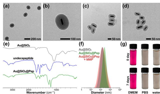
**Fig. 1** (a–d) TEM images of Au@SiO<sub>2</sub>@Pep (a and b) before and (c) 12 h and (d) 24 h after being incubated with MMP protease. (e) FT-IR spectra of YY-modified Au@SiO<sub>2</sub>, undecapeptide YYDPLGLADYY, and Au@SiO<sub>2</sub>@Pep. (f) Results of DLS of Au@SiO<sub>2</sub>@Pep before and after being incubated with MMP, compared with the results for Au@SiO<sub>2</sub>. (g) Photographs of Au@SiO<sub>2</sub>@Pep dispersions stored in DMEM, PBS, and water for 0 and 7 days.
